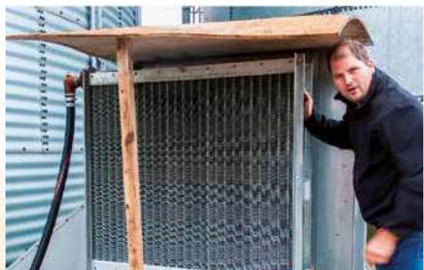
The air heater raises the outdoor temperature by 14 degrees and last year we had the grain dried down from 18.8 to 15 percent water in 10 days. "Quite a bit of straw was used in those days," says Morten Vilsgaard.
