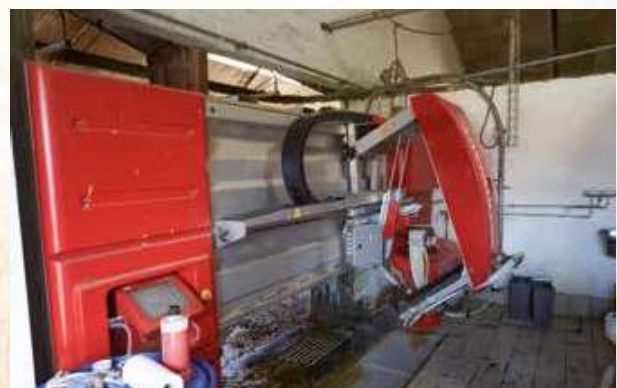
The milk robot is cleaned with 90 degree hot water.
